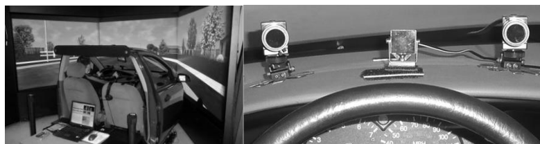
Figure 1. a) Driving simulator and b) eye tracker on dashboard
