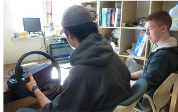
**Figure 2. Participant (left) and experimenter. The participant's left hand is placed on the steering wheel, with his fingers on the FSRs.**
