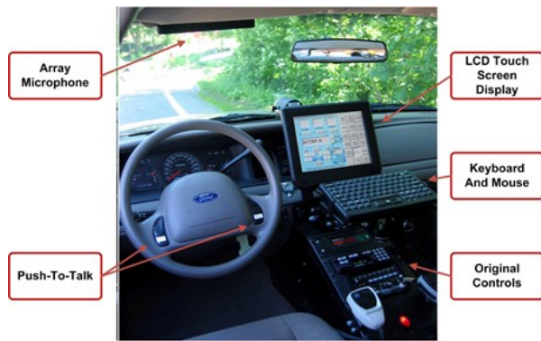
Figure 1. A typical Project54 system installation in a New Hampshire State Police cruiser. The user interface includes three parallel modes of operation: a noise canceling array microphone with steering wheel mounted push-to-talk; a 10 inch diagonal touch screen display with keyboard; and the original device control head controls.
